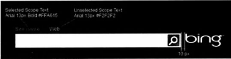
Redlines - Site Search Scopes Above the Searchbox with Reverse Color, Logo Right
