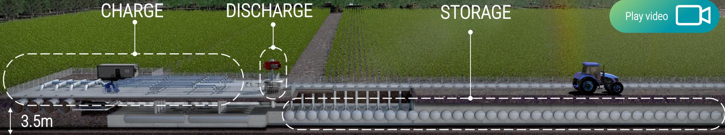
Separate charge, discharge and storage components enable multiple energy storage services
